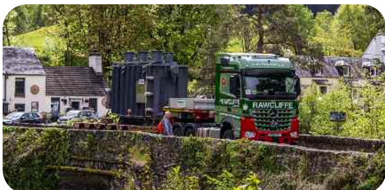
The new transformer for the refurbishment of the Glen Lochay power station passing over the Dochart Bridge
